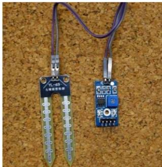
Gambar 3. Soil Moisture Sensor
